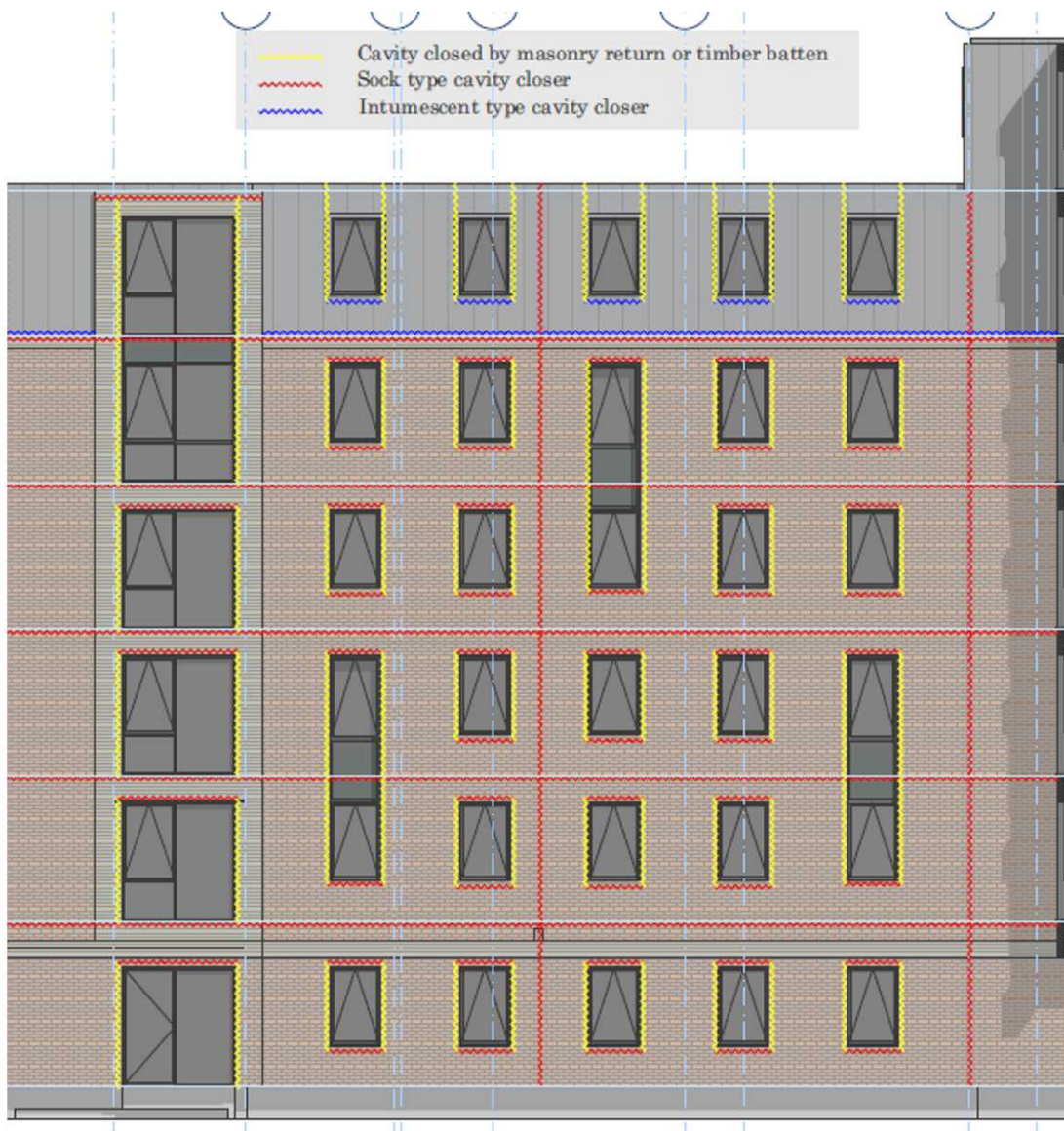
Figure 2 – Illustration of provision of cavity barriers behind cladding including around window and door openings.
